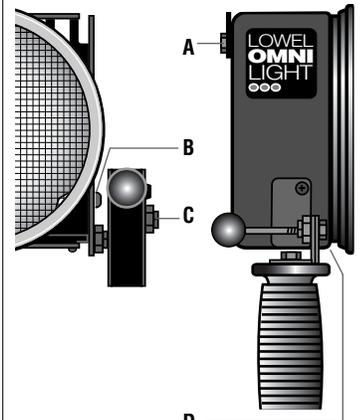
Omni has four constant-tension (torque) pivot points. All have flat spring washers to maintain proper tension and can be adjusted, if necessary, with a 7/16" wrench.
