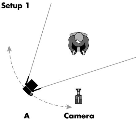
These 3 setups show some ways the Omni can be used; alone, with Tota-brella, or with diffusion, in a small lighting setup. Position of the lights and distance to the subject can be varied for different creative results. Varying the distance of either light from the subject will vary the contrast ratio between Key & Fill lights. **Tip:** position your subject away from walls to avoid shadows and give more a sense of depth.
