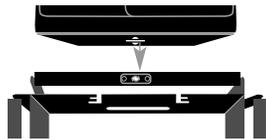
turn to remove or install doors. If barndoor frame fails to maintain proper tension on light, the frame should be removed and squeezed inward, very slightly.
