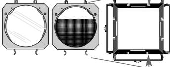
should be positioned in rear slots. Second accessory or snoot can then be used in forward slots.
