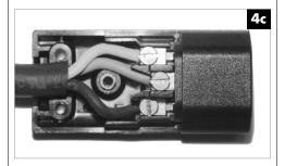
Place the conductors into terminal holes as shown, with White wire to **N**, Black wire to **L**, and Green wire to **Center**. Install & tighten the Green wire last. Tighten all firmly. After tightening, position the Green wire so it clears center screw post.
