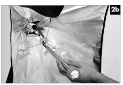
Take the new eXchange core and thread its power cable through the Rib Collar and Frame Tube, so that it appears out the back of the light. Push the core into place, seating the Rib Collar directly behind the base of the new core, so the Rifa shell is fully opened.
