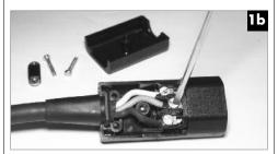
Using a flat head screwdriver, disassemble the power cord's IEC Connector, and remove the wires from their terminals. Slide rubber strain relief sleeve from power cord. Discard old IEC Connector
