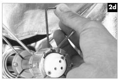
Using the supplied Allen Wrench, re-tighten the Set Screw in the Rib Collar firmly. If more tightening leverage is needed, use the other end of the wrench.
