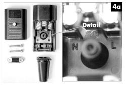
Disassemble the new IEC Connector completely by removing its Cover, Plug Strain relief, & 2 screws holding the Strain Relief Bar. Note that inside the IEC Connector, one screw is labeled **N** and the other is labeled **L**. Center screw is Ground (see Detail).
