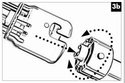
Line up the J-hook cutouts on the side of the lamphead with the side pins on the core. Note that 1 pin is larger than the other. Push & twist to install the removable lamphead on the core. When complete, remove Rifa from stand to wire the new IEC connector.
