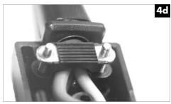
Slide the IEC Strain Relief along the cable and return it to its cutout channel in the IEC Connector. Replace the Strain Relief bar and tighten firmly.
