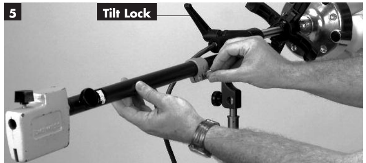
5 First slightly loosen Tilt Lock on SoftCore (arrow). Then loosen extension collar lock on Half Pole. Extend Half Pole carefully to get a working balance of the SoftCore, lamphead/lamps, and Pole counter-balance on stand. Tighten Tilt Lock on SoftCore, and lock Collar Knob on Half Pole. Note: be prepared to adjust balance after adding the softbox.
