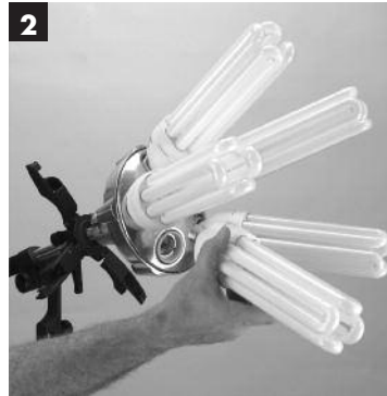
2 Carefully install all fluorescent lamps by holding them at their base.
