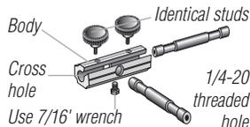
**The three main parts of the Interlink can be used together or separately.**
