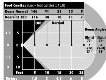
Beam angles-points at which intensity drops to 50% of maximum
