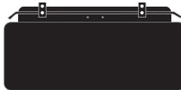
**Side Shades** can be used only when top and bottom panels are attached. Turn each black clip 45° and attach one each to the bent rod ends of the top and bottom panels. Reflector doors must be held tightly against their 45° angle stops while doing this.
