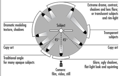
The oversimplified diagram above shows some of the ramifications of positioning lights for different subject types & lighting effects. The diagram is only useful as a starting point for new pros. All subjects & scenes are different and make different demands upon lighting. The height of the lights & camera, and the subjects angles & reflectivity must be considered.
