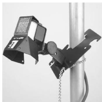
The Home-plate allows the mounting of L-lights on floors and other horizontal surfaces, on pipes and stand shafts, behind moldings, and, with Lowel Gaffer-tape, to windows and some vertical surfaces. Always position Home-plate with the large & small mounting notches on top and chain lock slots on the bottom.
